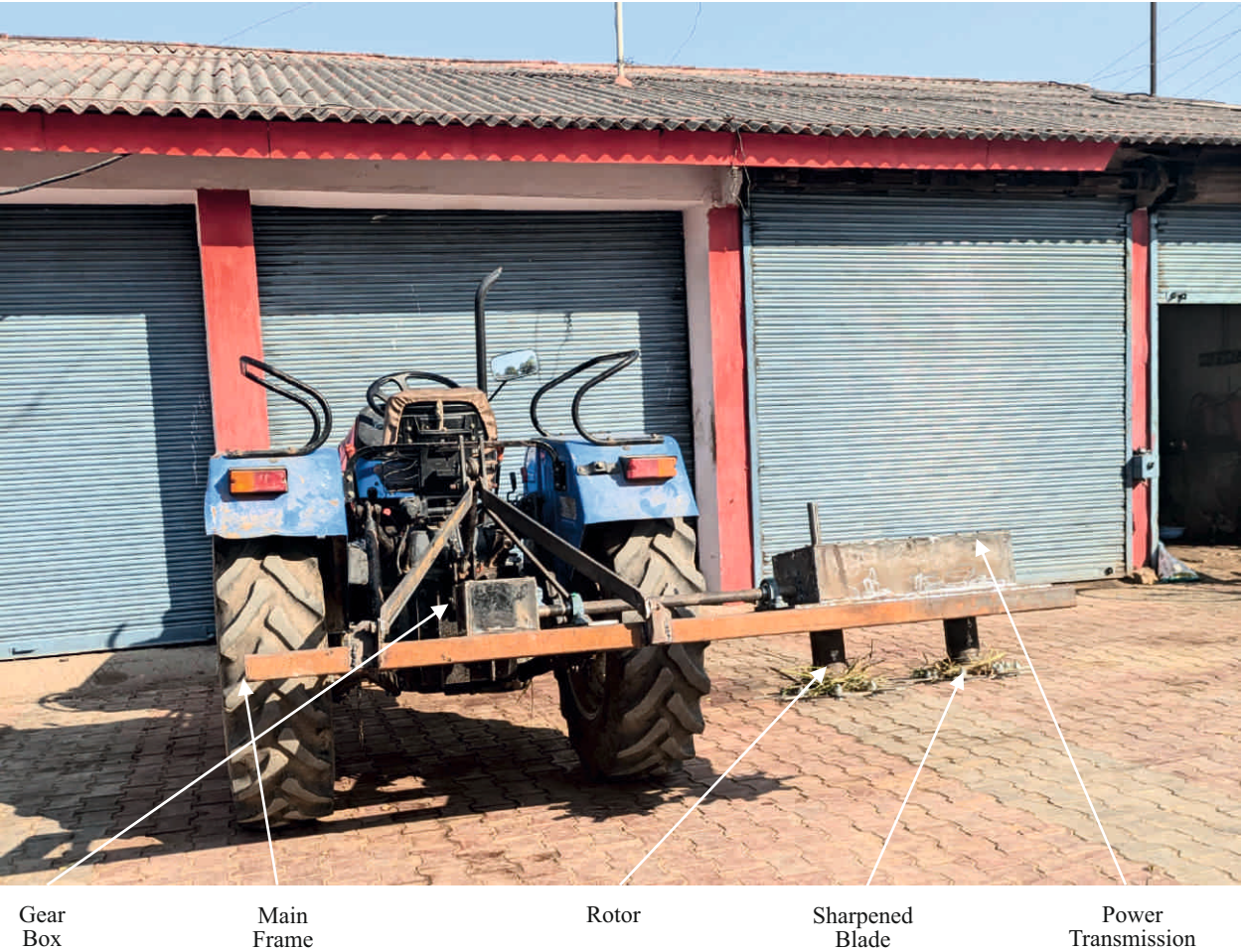
Fig. 3.5.4. Prototype of the developed BN hybrid forage harvester
